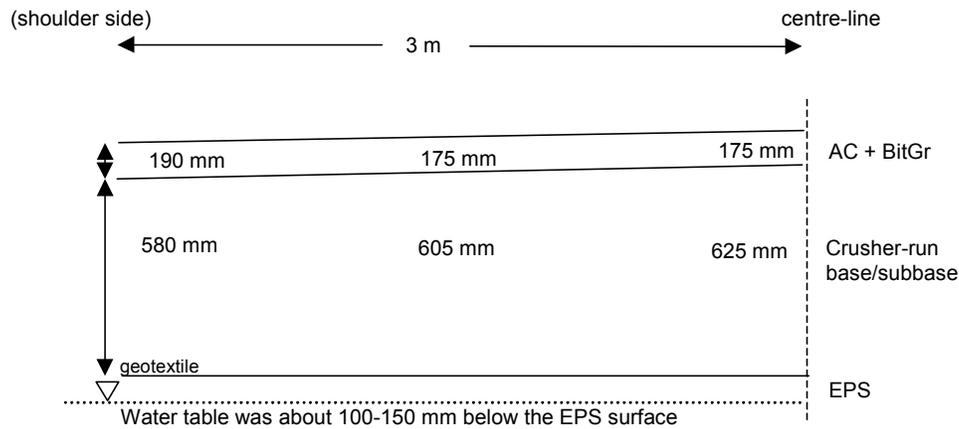
Figure 2. The measured thickness of layers in the trial pit.
