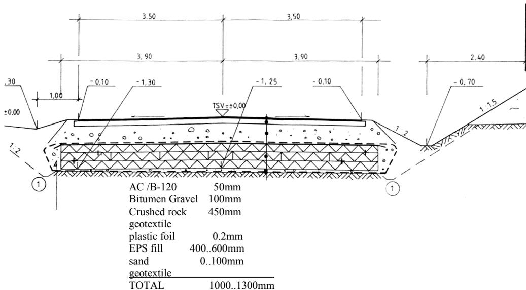
Figure 1. The design of EPS-filled street section of Pesurinkatu-street in Vammala (1986).
