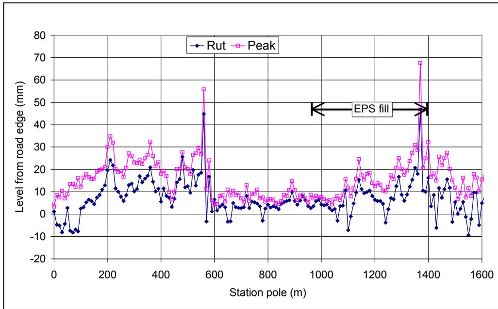
Figure 7. Rut and peak values on Pesurinkatu. Values were measured with the Finnish road surface monitoring system (PTM). The differences between measured peak and rut describe transverse unevenness of road profile.
