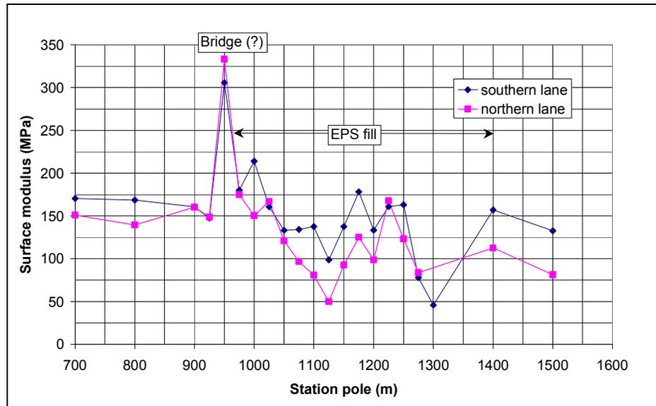
Figure 4. Measured surface modulus on Pesurinkatu in 28 October the 28<sup>th</sup>, 1999.
