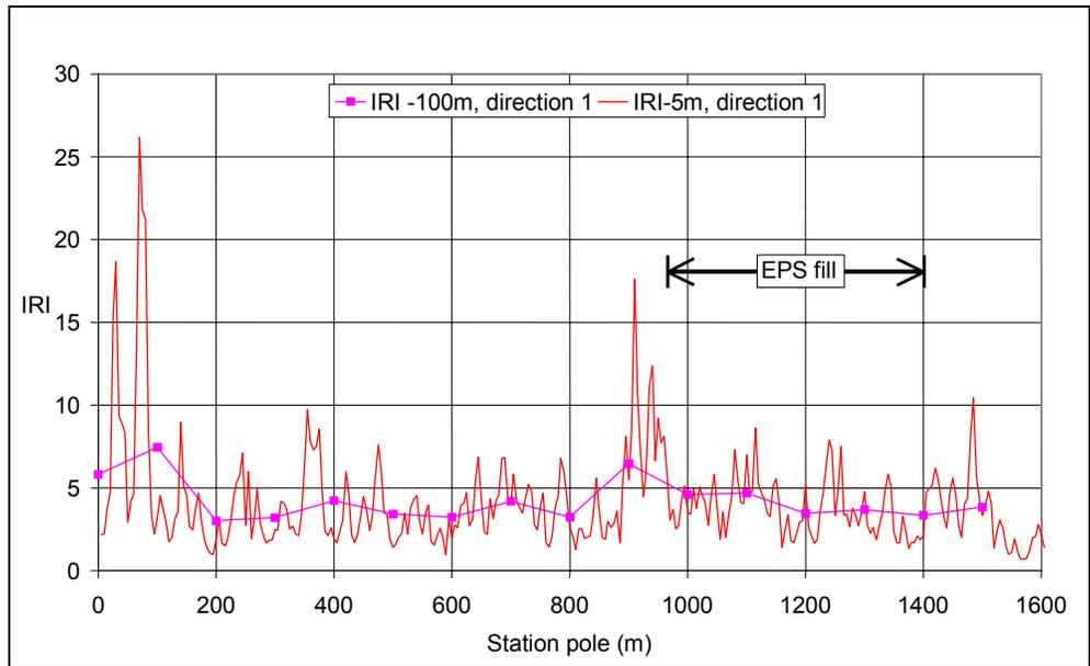
Figure 5. Measured IRI-100m and IRI-5m values, direction 1 (Northern lane).
